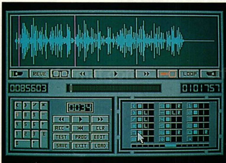
■ The sequencer can be conjured up from the main display and allows you to program up to 18 samples into the keypad keys. These may then be replayed in any order you like. The letters next to the programmed keys indicate whether the sample will loop or be played in reverse.
